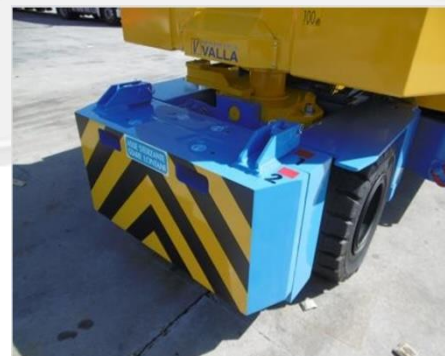
Removable ballasts to make it easier to transport the crane
