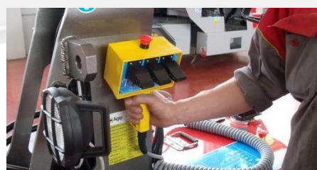
Wired remote control for the aerial part
