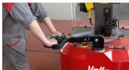
180° steering helm powered by electric motor with 180° rotation for maximum manoeuvrability
