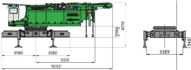
5500 E basic machine with star-lifter tele-undercarriage and with lower boom
