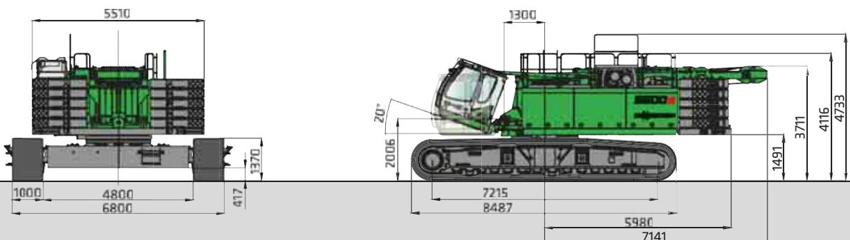
5500E basic machine without lower boom section and with circumferential railing\*
