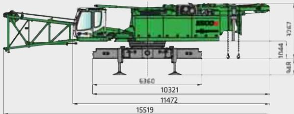
5500 E basic machine with star-lifter tele-undercarriage without lower boom
