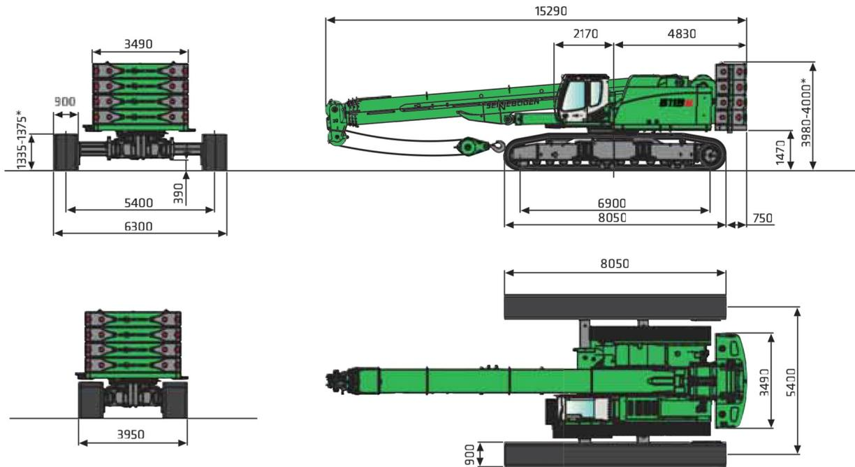
Weight: approx. 79.7 t (2 winches, 8 m fly jib, 80 t hook, no counterweight, 900-mm triple-bar-shoes)
