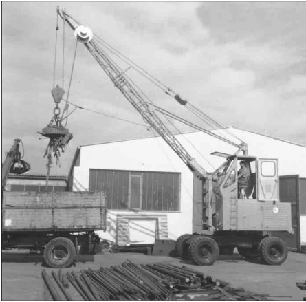
1962: Rope-driven S833 with elevated operator cab
