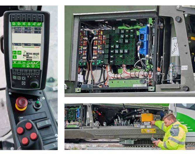
The SENCON control system supports you with diagnostics and makes troubleshooting easier. So your machine is back in action more quickly. All maintenance and service points are arranged clearly and easily accessible. The clear labeling of components makes finding your way around easy.
