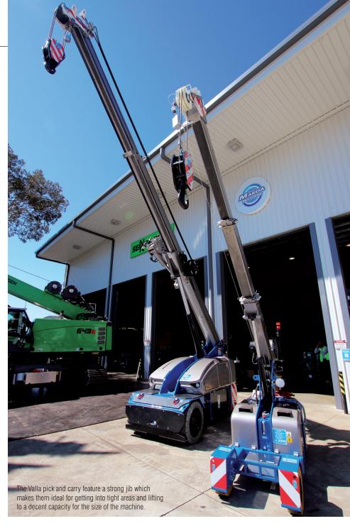
remote-controlled machine which has led to a more compact and manoeuvrable model. The older models featured a cab for the operator or controls on the back of the machine to steer it around, which limited the scope of works for the machine.
