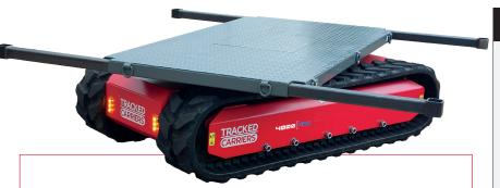
The new 4000 PRO from Tracked Carriers offers an unrivalled method of transporting heavy goods through confined spaces. At only 1m wide, the 4000 PRO has a maximum capacity of 4,000kg and can climb gradients up to 45° with a reduced load.
