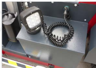
» LED working spotlight with magnetic base
