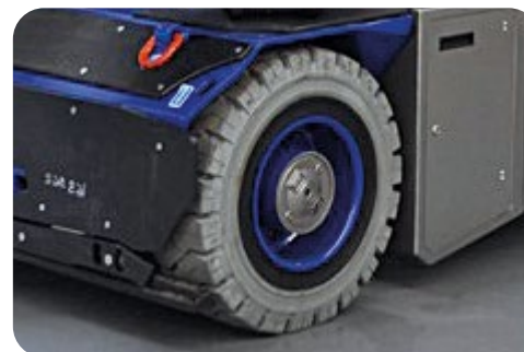
RUOTE ANTISTRACIA Non-marking tires / Roues non marquant Non-Marking-Räder / Ruedas anti-marcas
