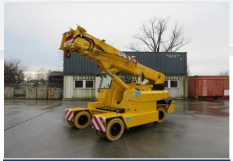
Hydraulic jib that can be turned on the boom side when not used
